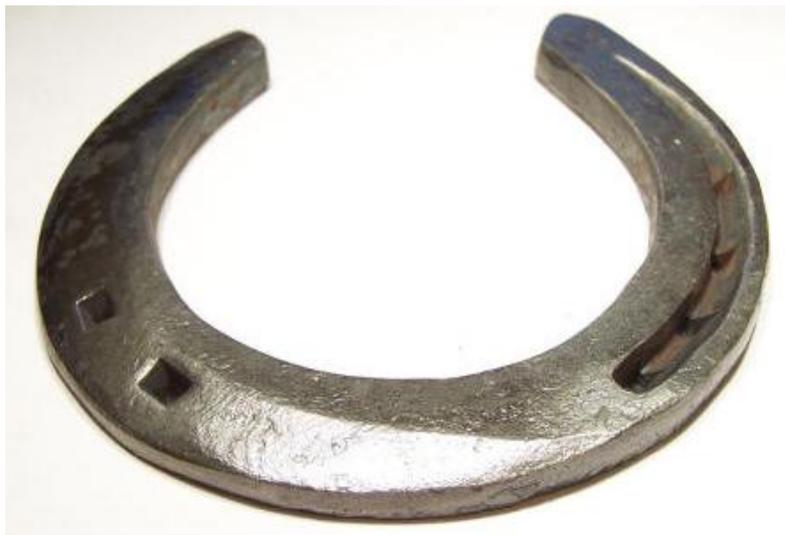
The toe is bent and the outside branch formed. The outside branch is then chamfered on the ground surface towards the outside, retaining the thickness of the inner edge. The chamfering, which has the effect of broadening the web, should be greatest at the heel and gradually reduced towards the toe.
